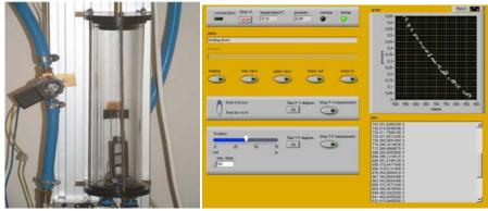
Fig.2: A remote experiment on phenomenological thermodynamics. Left: A piston compresses air in a glas cylinder. A heater (below) controls the temperature of the air. Pressure and temperature are measured by the PC. Right: The LabView user interface of this experiment.
